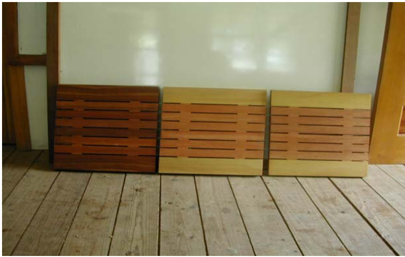
19. Floor samples (Cumbillo [ Terminalia amazonia ] and selillon [ Pouteria izabalensis ]/left; huesito [ Macrohassltia macrotherantha ] and Piojo [ Tapiriria guianensis ]/center; varillo [ Simphonia glubulifera ] and San Juan Rojo [ Vochysia sp]/right). COATLAHL Cooperative, La Ceiba, Atlantida, Honduras.
